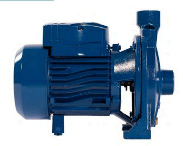
The pump is mainly composed of three parts: motor, water pump and seal. A single-end mechanical seal is installed between the water pump and the motor. "O"-shaped oil-resistant rubber sealing ring is used for static sealing at the sealing part of the fixed stop.
